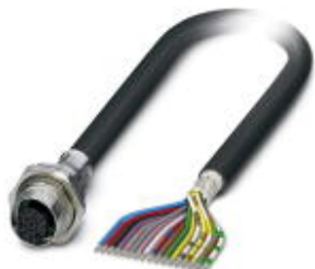
Flush-type socket, shielded, 17-pos., M12, A-coded, rear/screw mounting with M16 thread, with 1 m cable, 17 x 0.14 mm 2
