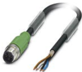
Sensor/Actuator cable, 4-position, PUR halogen-free, black-gray RAL 7021, shielded, Plug straight M12, A-coded, on free cable end, Cable length: 10 m
