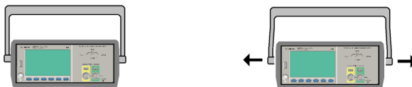
To remove the handle, rotate it to the vertical position and pull the ends outward.
