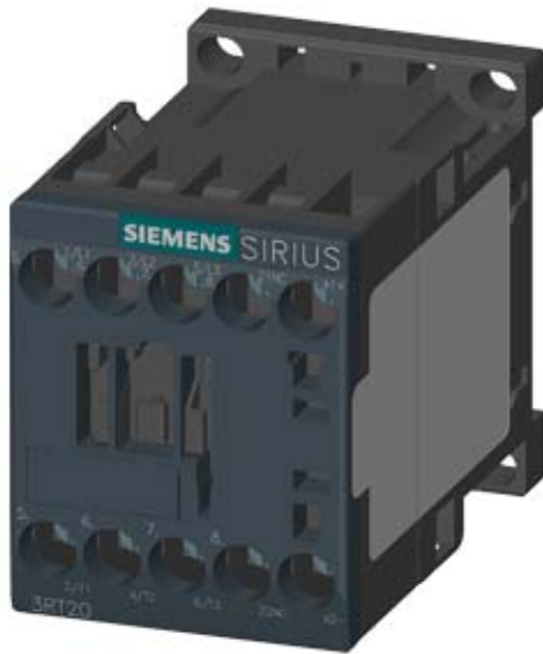
CONTACTOR, AC-3, 4KW/400V, 1NC, DC 24V, 3-POLE, SZ S00 SCREW TERMINAL
