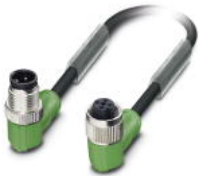
Sensor/Actuator cable, 3-position, PUR halogen-free, black-gray RAL 7021, Plug angled M12, A-coded, on Socket angled M12, A-coded, PIN 2+4 bridged, Cable length: 0.6 m
