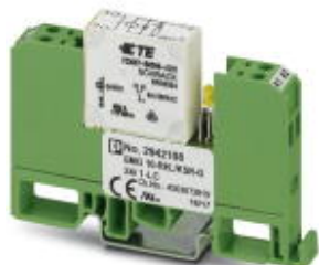
Relay module, with soldered-in miniature switching relay, contacts (AgNi): Medium to large loads, 1 N/O contact, input voltage 24 V DC
