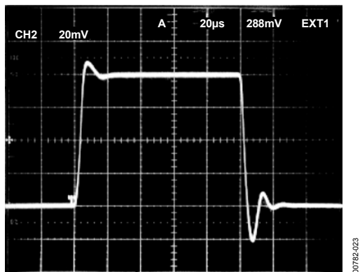
Figure 25. Small Signal Pulse Response, G = +5 , R_L = 20 \text{ k}\Omega , C_L = 50 \text{ pF}
