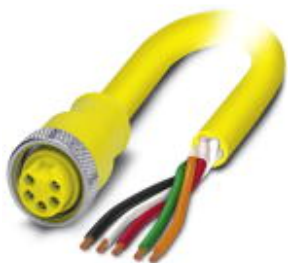
Sensor/Actuator cable, 5-position, PVC, Yellow RAL 1021, free cable end, on Socket straight 7/8"-16UNF, A-coded, Cable length: 4 m
