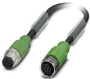
Sensor/Actuator cable, 8-position, PUR halogen-free, black-gray RAL 7021, shielded, Plug straight M12, A-coded, on Socket straight M12, A-coded, Cable length: 3 m
