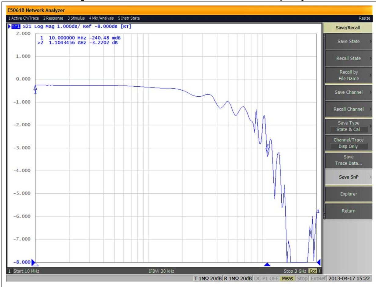
Figure 22. Data switch transfer characteristics vs. frequency
