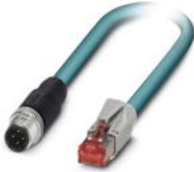
Assembled Ethernet cable, CAT5e, shielded, 2-pair, AWG 26 stranded (7-wire), RAL 5021 (water blue), M12 plug on RJ45 plug/IP20, line, length 2 m
