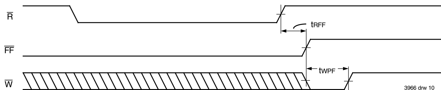
Figure 8. Minimum Timing for an Full Flag Coincident Write Pulse
