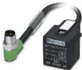
Sensor/Actuator cable, 3-position, PUR halogen-free, black-gray RAL 7021, Plug angled M12 SPEEDCON, A-coded, on Valve connector A, with 1 LED, connected with Z diode, Cable length: 3 m
