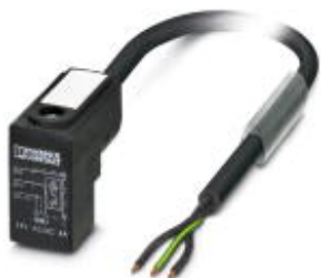
Sensor/Actuator cable, 3-position, PUR halogen-free, black-gray RAL 7021, free cable end, on Valve connector C (8 mm), with 1 LED, connected with Varistor, Cable length: 3 m
