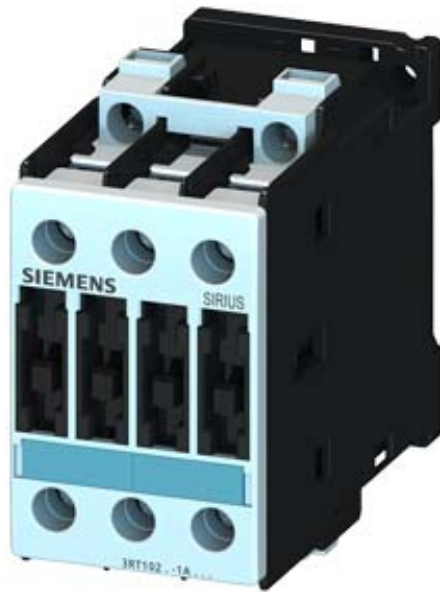
CONTACTOR, AC-3 5.5 KW/400 V, AC 230 V, 50 HZ, 3-POLE, SIZE S0, SCREW CONNECTION
