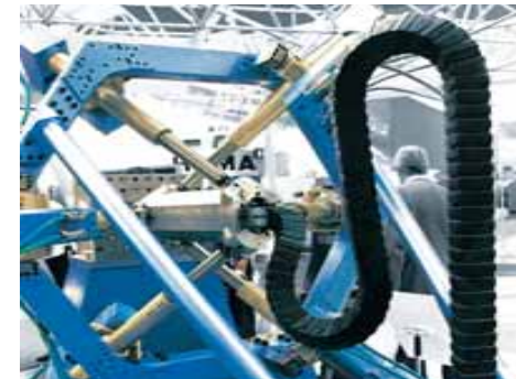
triflex® for 3 movement directions combined with triflex® for 1 movement direction
