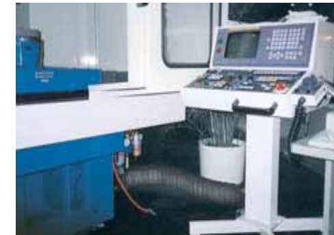
triflex® 332 as unsupported link from machines to control desk
