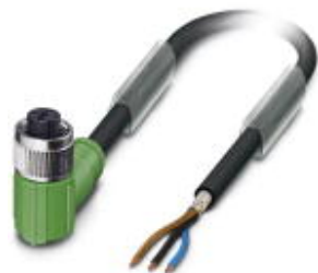
Sensor/Actuator cable, 3-position, PUR halogen-free, black-gray RAL 7021, shielded, free cable end, on Socket angled M12, A-coded, Cable length: 10 m
