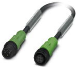
Sensor/Actuator cable, 4-position, PUR halogen-free, black-gray RAL 7021, Plug straight M12, A-coded, on Socket straight M12, A-coded, Cable length: 3 m, with plastic knurl
