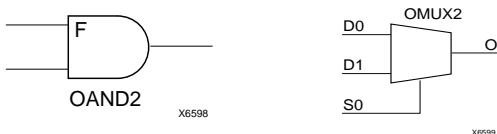
Figure 7: AND & MUX Symbols in Spartan-XL IOB
