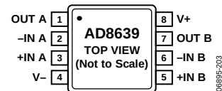
Figure 3. 8-Lead MSOP (RM-8) 8-Lead SOIC_N (R-8)
