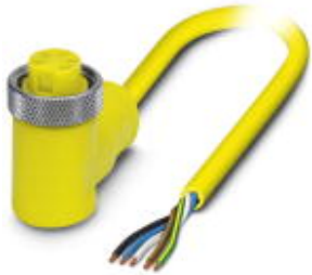
Sensor/Actuator cable, 5-position, PVC, Yellow RAL 1021, free cable end, on Socket angled 7/8"-16UNF, A-coded, Cable length: 2 m
