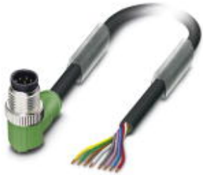
Sensor/Actuator cable, 8-position, PUR halogen-free, black-gray RAL 7021, Plug angled M12, A-coded, on free cable end, Cable length: 10 m
