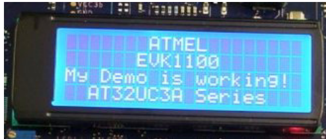
Figure 6-50. LCD Display showing edited message
