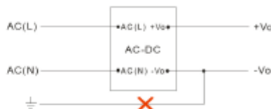
(Figure 2): This application is not available for this series. Note: If you have such application, please consult to our FAE department.
