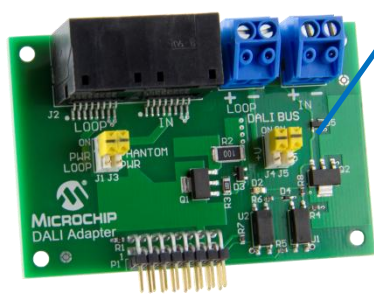
DALI Adapter with 2-wire & RJ45 connections
