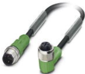
Sensor/Actuator cable, 3-position, PUR halogen-free, black-gray RAL 7021, Plug straight M12, A-coded, on Socket angled M12, A-coded, PIN 2+4 bridged, Cable length: 3 m
