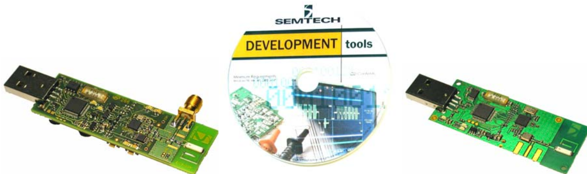
Figure 3: SX1230-11SKA Contents (CR2032 Cell not Shown)
