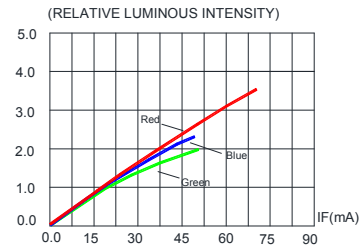
FIG.2 RELATIVE LUMINOUS INTENSITY VS. FORWARD CURRENT
