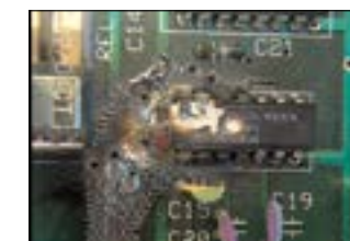
Figure 4. Damage occurs when a transient overvoltage exceeds the withstand voltage of electrical and electronic equipment.
