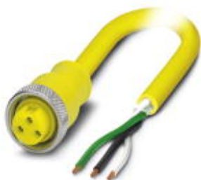
Sensor/Actuator cable, 3-position, PVC, Yellow RAL 1021, free cable end, on Socket straight 7/8"-16UNF, A-coded, Cable length: 4 m
