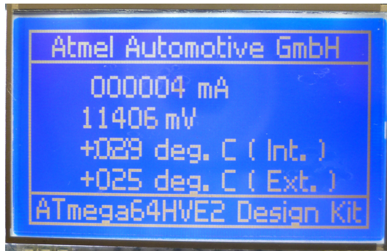
Figure 4-2. Instantaneous Measurement Values on the LCD Display of the LIN Master Unit
