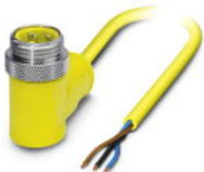
Sensor/Actuator cable, 3-position, PVC, Yellow RAL 1021, Plug angled 7/8"-16UNF, A-coded, on free cable end, Cable length: 2 m
