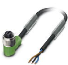
Sensor/Actuator cable, 3-position, PUR halogen-free, Black-gray RAL 7021, Free cable end, on Socket angled M12, A-coded, Cable length: 5 m
