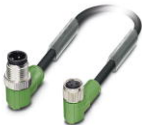
Sensor/Actuator cable, 3-position, PUR halogen-free, black-gray RAL 7021, Plug angled M12, A-coded, on Socket angled M8, Cable length: 0.3 m
