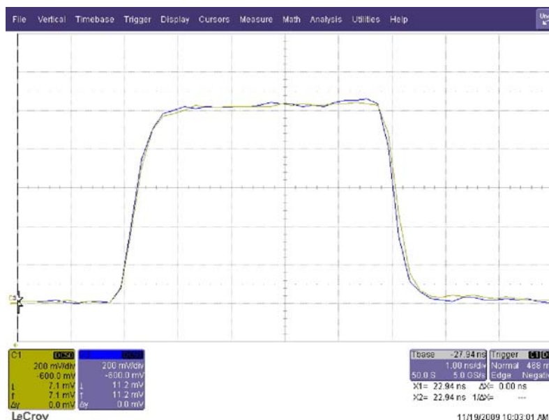
Figure 9. Scope Plot - De-skewed Outputs
