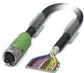
Sensor/Actuator cable, 17-position, PUR/PVC, Black RAL 9005, shielded, free cable end, on Socket straight M12 SPEEDCON, A-coded, Cable length: 10 m
