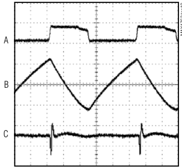
LIGHT-LOAD SWITCHING WAVEFORMS
