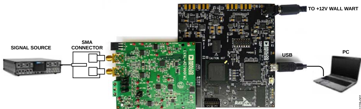
Figure 1. Setting Up the EVAL-AD7960FMCZ
